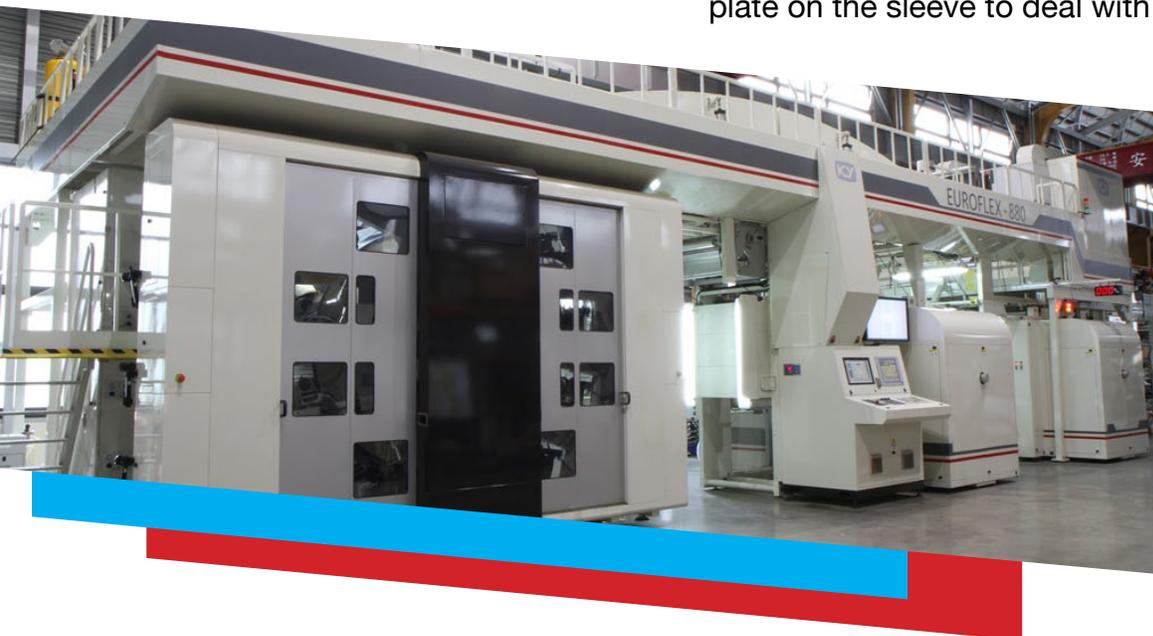
After conducting extensive engineering and print trials, a press that can answer the need for a mid-web press is now on the market: A 34 in. (860 mm.) 8- and 10-color all servo CI press from KYMC. This machine has been engineered to meet the challenges of shorter runs and at the same time be able to run at high speeds to handle longer runs profitably. It is able to achieve gravure print quality
