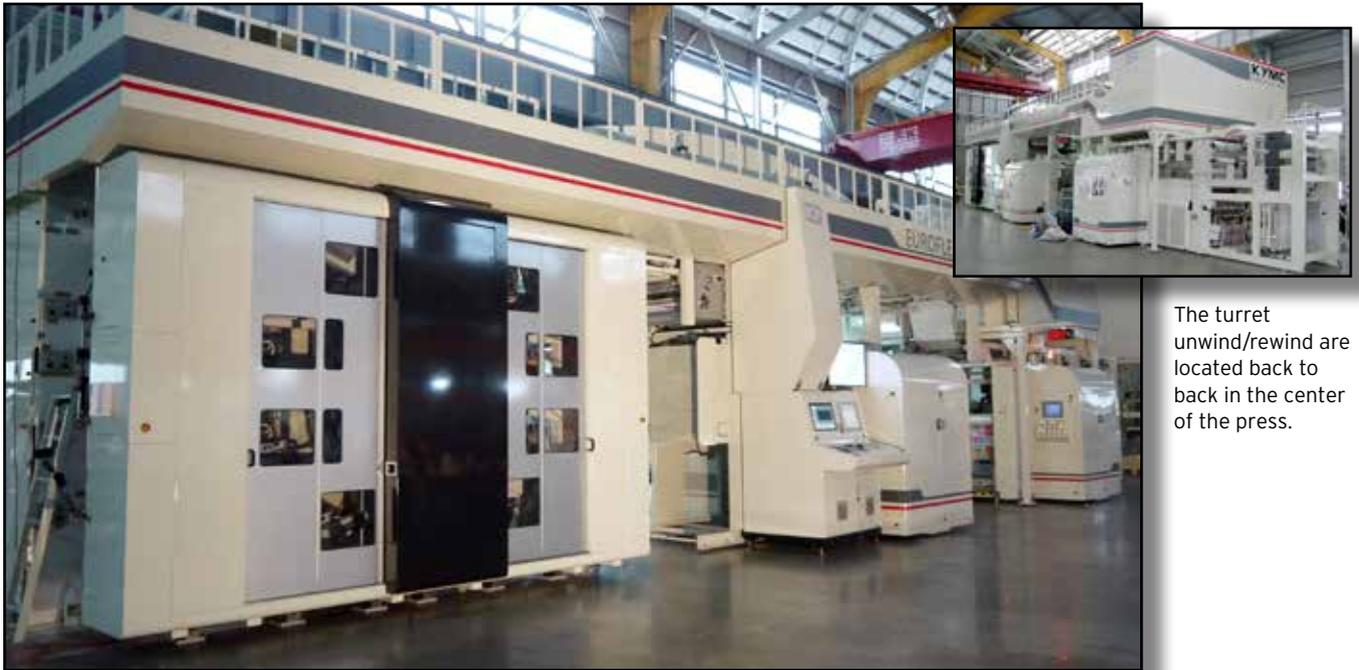
The turret unwind/rewind are located back to back in the center of the press.
